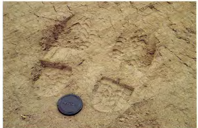
On a properly roller packed site – a footprint barely registers.
