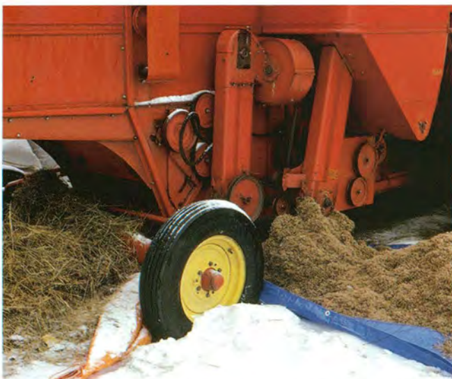
Here little bluestem with large amounts of straw is being dropped through a trap door in the back of this Massey Ferguson 300 combine. The elevator chain has been removed so that seed does not travel up into the grain tank, but augers out onto a tarp on the ground. This set up removes most of the large straw from the seed. From here it will now go to a de-bearder to break up the remaining small straw.
