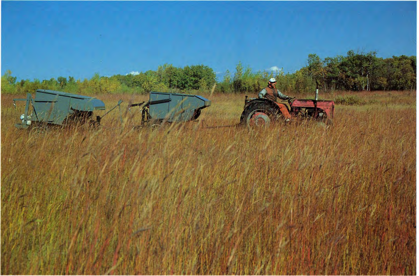
Pull type native seed strippers are able to collect large volumes of diverse native seeds efficiently with minimal impact on the native prairie.
