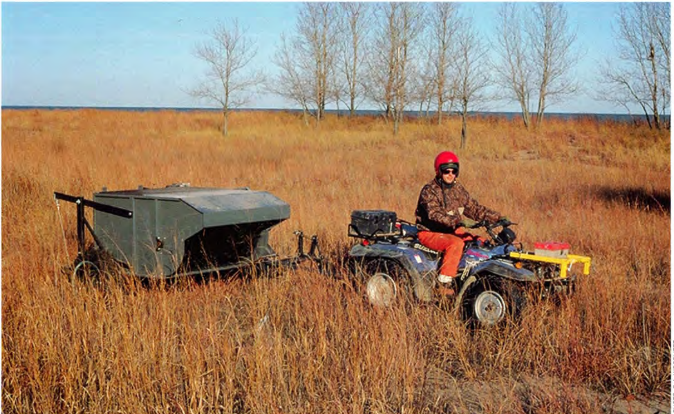
Pull type seed stripper harvesting little bluestem on a tall grass prairie in SW Ontario.
