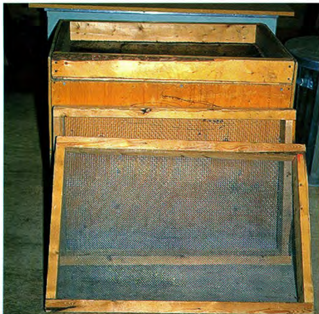
A series of screens can be made from various guages of screen or hardware cloth. Make wooden frames to fit the screens and construct a box to fit the frames into.
