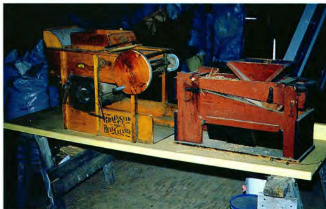
Small fanning mill (left) and blanket cleaner (right) are useful for cleaning native seed.
